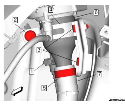
2. Remove the fuel tank filler pipe (6) from the vehicle. Refer to *Fuel Tank Filler Pipe Replacement* in SI.
