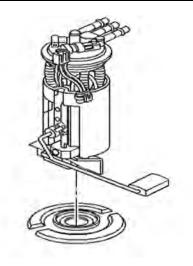
4. Install the new fuel pump module. Refer to Fuel Tank Fuel Pump Module Replacement in SI.
