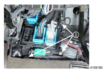
9. If temporarily secured, disconnect the junction block from brake pedal, reposition to firewall studs and install the retaining nuts (1). Tighten the nuts to 9 N\*m (80 lb in).
