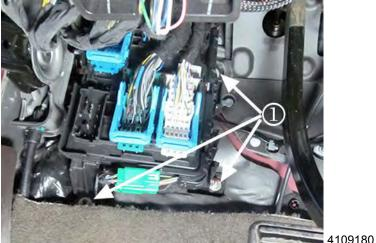
2. Remove the three nuts retaining the junction block assembly (1).
