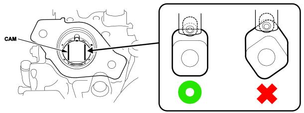
8. Lubricate the cam and roller with clean engine oil, and then install the high pressure fuel pump with the new fuel line clip. Loosely install the bolts.
