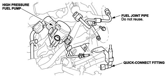
Remove the high pressure fuel pump.
