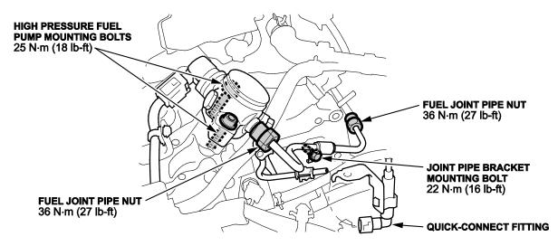
11. Reinstall the parts in reverse order, and then check for any fuel leaks.
