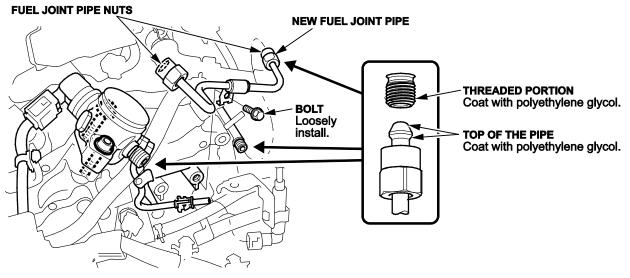
10. Torque the high pressure fuel pump mounting bolts and fuel joint pipe nuts to the specifications shown below.
