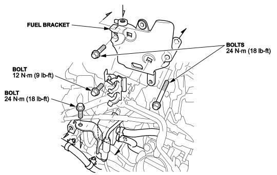
2. Remove the EVAP canister purge valve.
