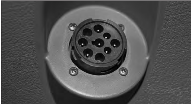
FIGURE 14 - TYPICAL VEHICLE DIAGNOSTIC CONNECTOR LOCATIONS (J1939)
