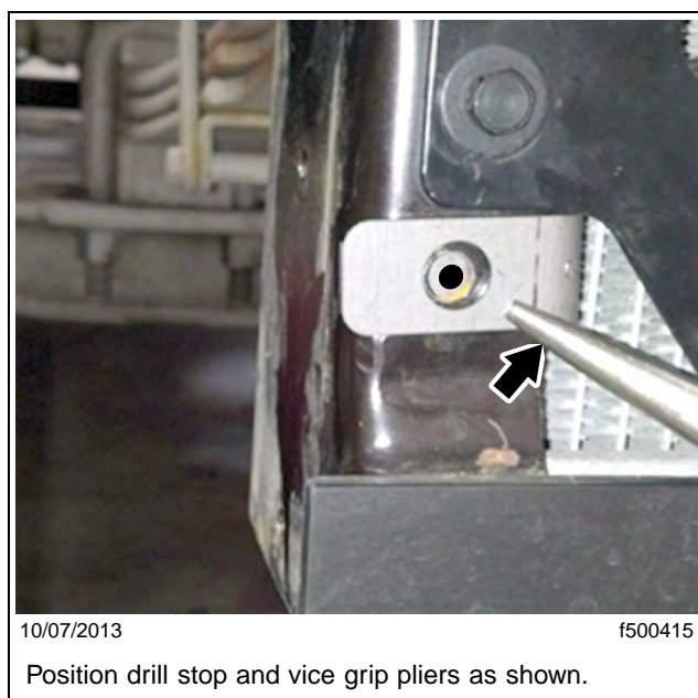
Fig. 4, Drill Stop Installation
