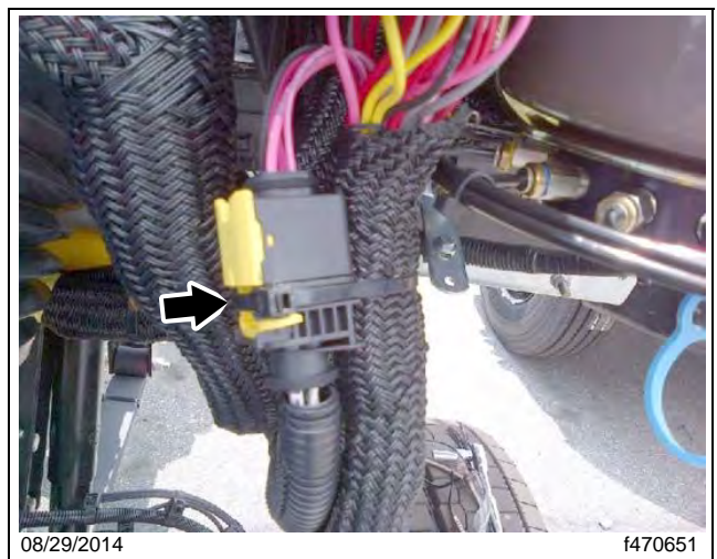
Fig. 12, Attaching the Connector
