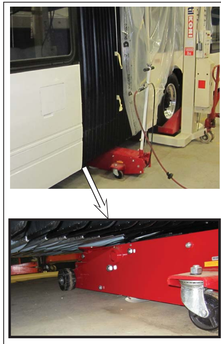
Figure 1 - Floor Jack Location Under the Vehicle to Support the Turntable
