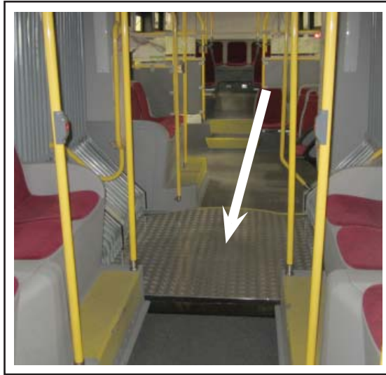
Figure 2 - Articulation Potentiometer Access Plate Location
