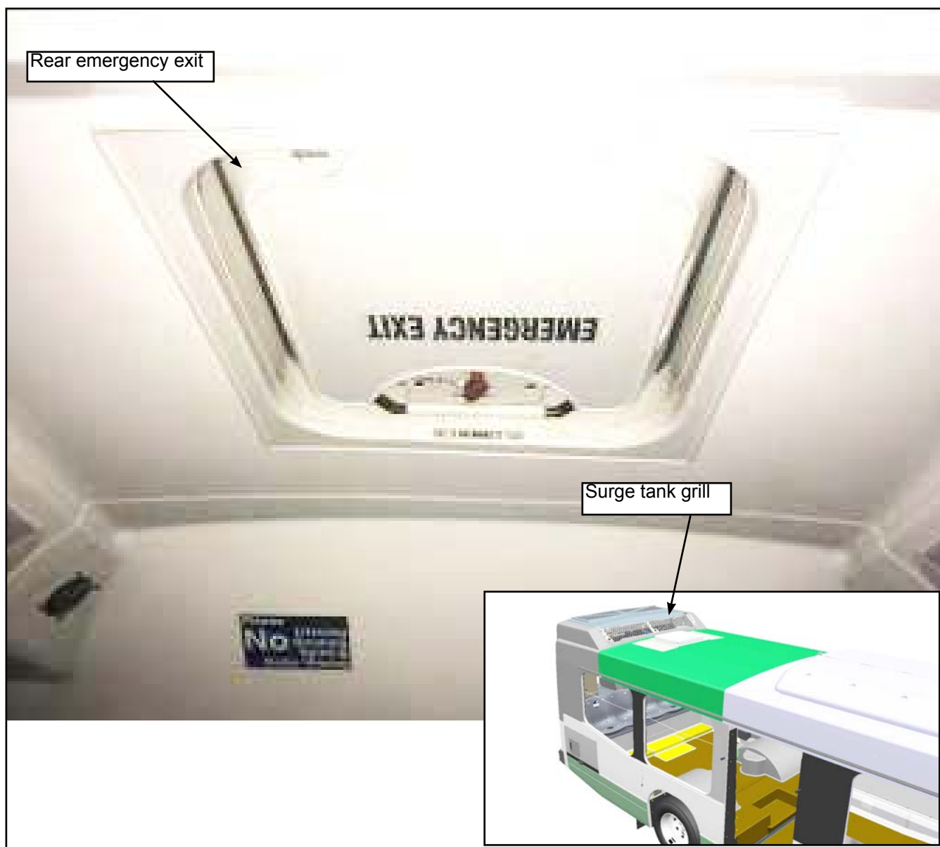
Figure 1 - Rear emergency exit and and surge tank grill on the roof
