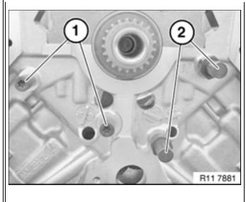
The current ISTA repair manual RA11 31 052 "Replacing both timing chains \ PREMIUM" instructs to release tension on four bearing bolts (indicated as #1 for cylinders 5 to 8; and #2 for cylinders 1 to 4) on the engine block.
