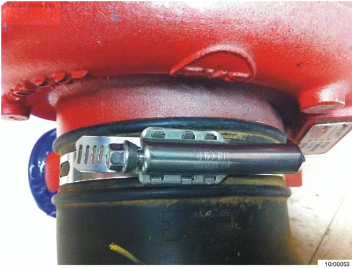
Figure 1: The gap indicating a clamp not at proper torque.
