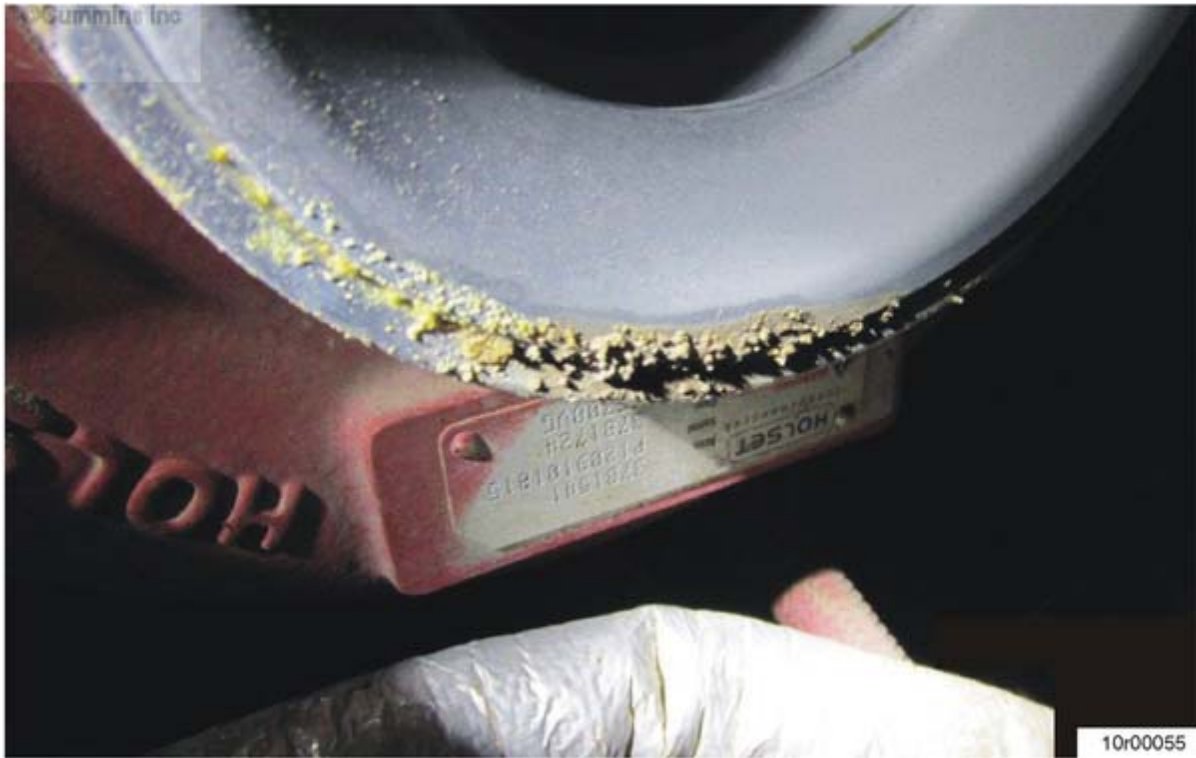
Figure 3: Buildup of dirt/debris at the 6 o'clock position on the turbocharger compressor inlet.
