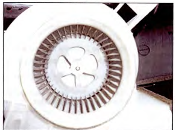
Figure 2. HV Battery Cooling Fan AFTER Cleaning
