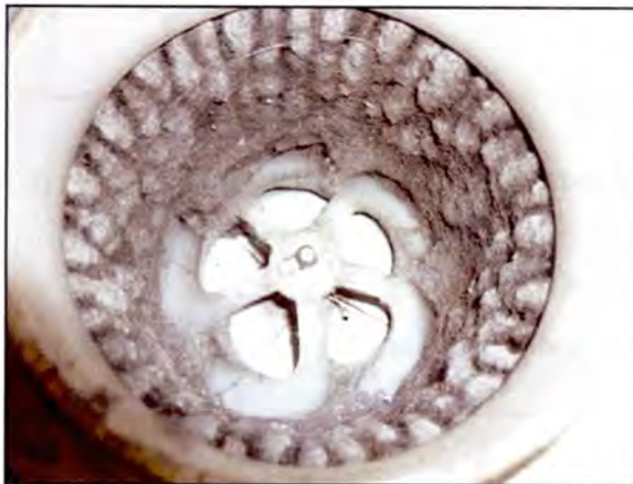
Figure 1. HV Battery Cooling Fan BEFORE Cleaning
