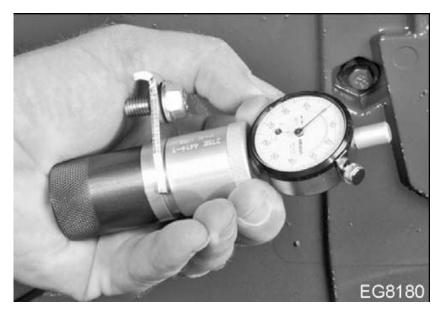
3. Remove the cam sensor and install the camshaft end play tool. Once the tool is installed rotate clockwise by hand 14 times and stop to zero out the tool. Next rotate the engine by hand 14 times counter clockwise and record the reading. The end play should be 0.005-0.013in, if it is higher than this the cam gear has walked off the camshaft.
