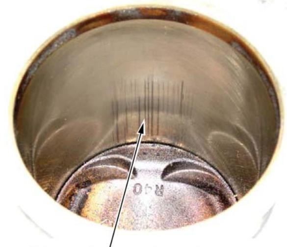
33. Remove the piston from the scratched cylinder bore. Inspect the piston skirt for any scratches or damage that corresponds with the scratched cylinder bore.
