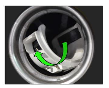
Insert the lockout mechanism into the filler neck and rotate from right-to-left <arrow> to seat properly into position.
