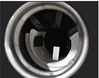
Align the lockout mechanism with the tabs in the filler neck, then push the lockout mechanism down into the filler neck until it is fully seated <as shown>.
