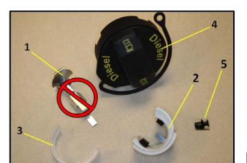
The misfueling guard kit p/n - 5K0 201 400 consists of five pieces (left) which must be installed in the following order:
