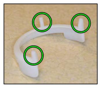
The retaining ring is installed into the filler neck with the alignment pins <circles> facing toward the fuel tank.
