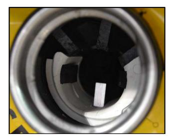
Align the lockout mechanism with the tabs in the filler neck, and then push the lockout mechanism down into the filler neck until it is fully seated <as shown>.
