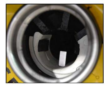
Align the lockout mechanism with the tabs in the filler neck, and then push the lockout mechanism down into the filler neck until it is fully seated <as shown>.
