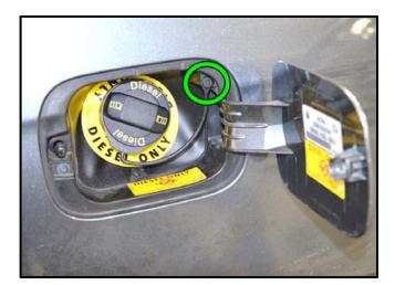
⇐ The retaining ring is installed into the filler neck with the alignment pins <circles> facing toward the fuel tank.
