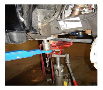
7. Using a transmission jack, align the exhaust pipe, downpipe and the turbocharger exhaust pipe flanges until all mounting joints and the flanges are flush and parallel with no or minimal load or force applied. This could include adjusting the mounts as necessary, allowing the flanges to sit flush with the exhaust in a neutral state, using care not to compromise clearances around the exhaust.
