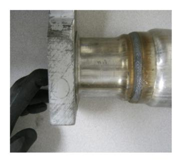
This can be inspected easily by placing a gauge block flush against the flange and inspect for excessive gaps or damage to the flange.
