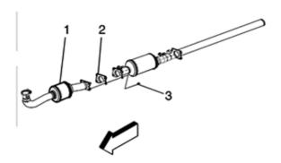
5. Loose or disconnect the four flange mid-joint bolts located after the catalytic converter.
