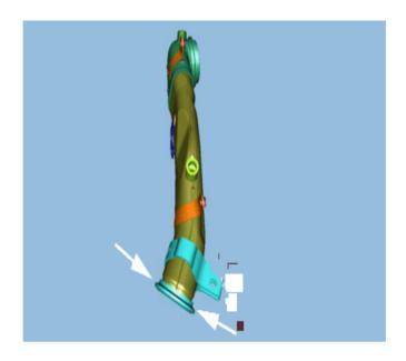
**Note:** The illustration above is the turbocharger exhaust pipe without a pilot flange.
