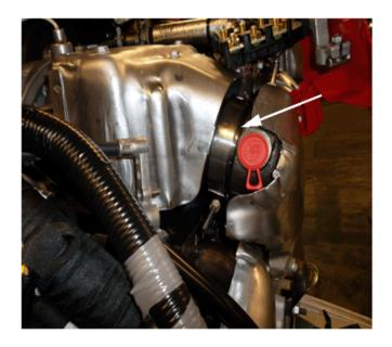
9. After alignment of all the joints, install and tighten a new clamp at the turbocharger (if removed earlier).
