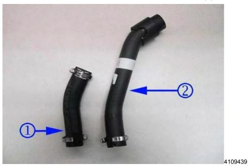
4.2 Match the new hose (2) to the original (1), aligning side by side.
