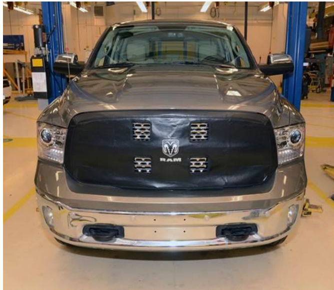
Fig. 3 Winter Front Cover Installed
