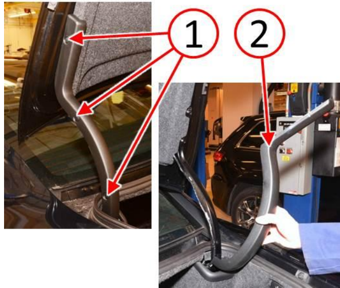
Fig. 5 Remove Hinge Covers
