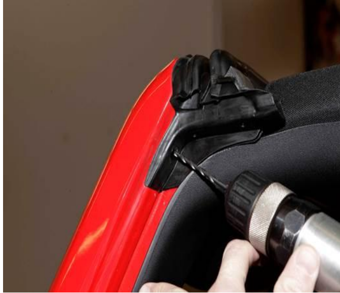
Fig. 2 Drilling out Rivet
