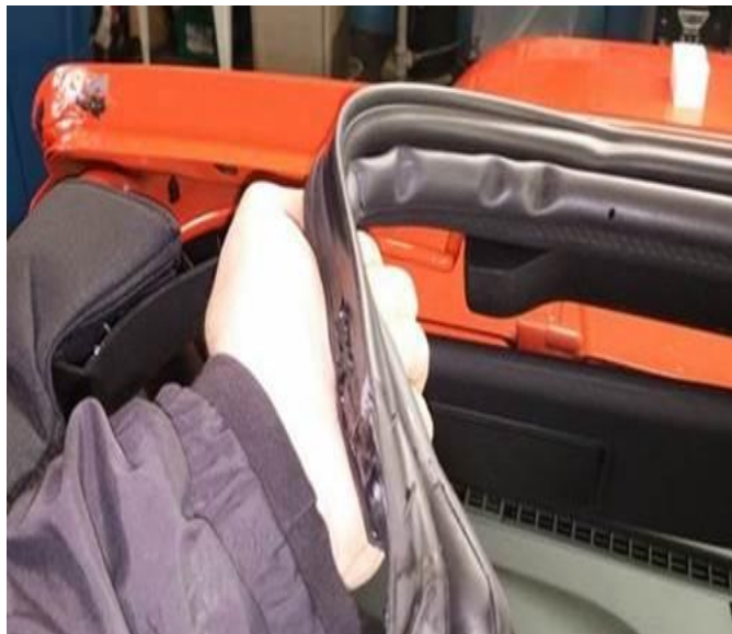
Fig. 4 Header Seal Removal
