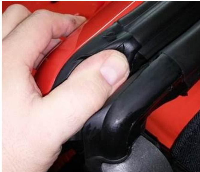
Fig. 21 Seal Corner Alignment
