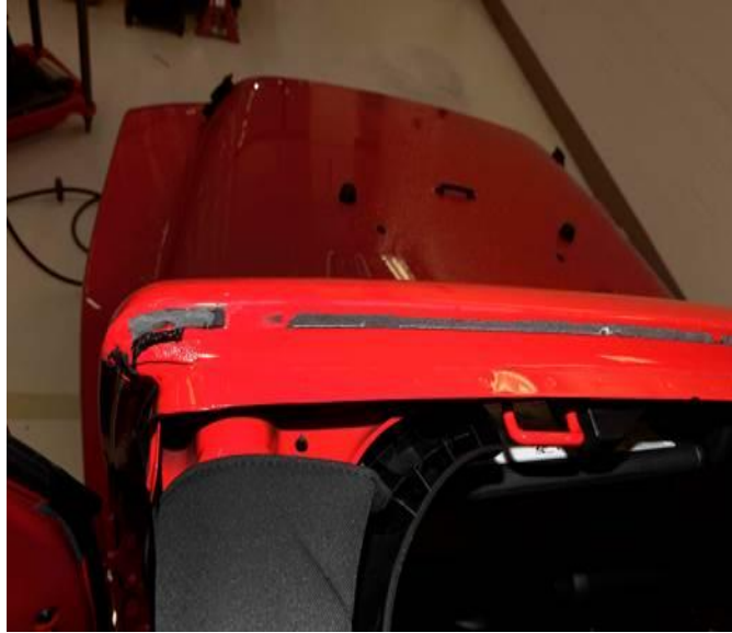
Fig. 5 Removing Residue Butyl
