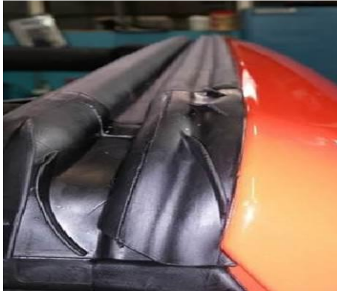
Fig. 27 Properly Aligned Seal
