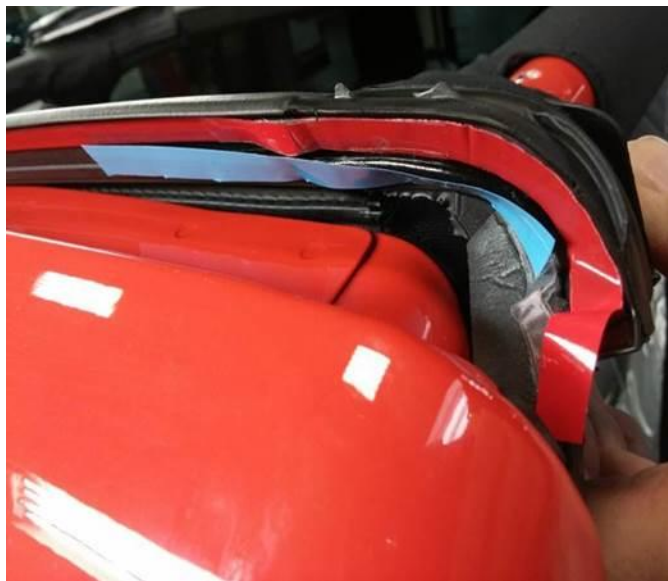
Fig. 15 Rocking The Seal In Place
