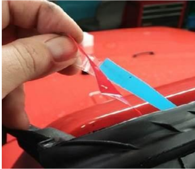
Fig. 16 Removing Adhesive Pulls
