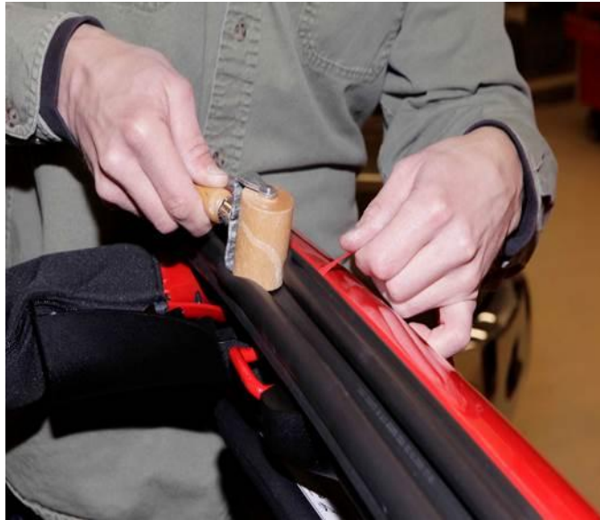
Fig. 24 Using Roller On Seal
