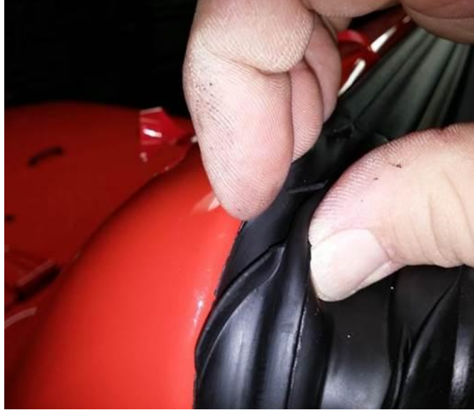
Fig. 20 Seating End Piece Seal At Frame
