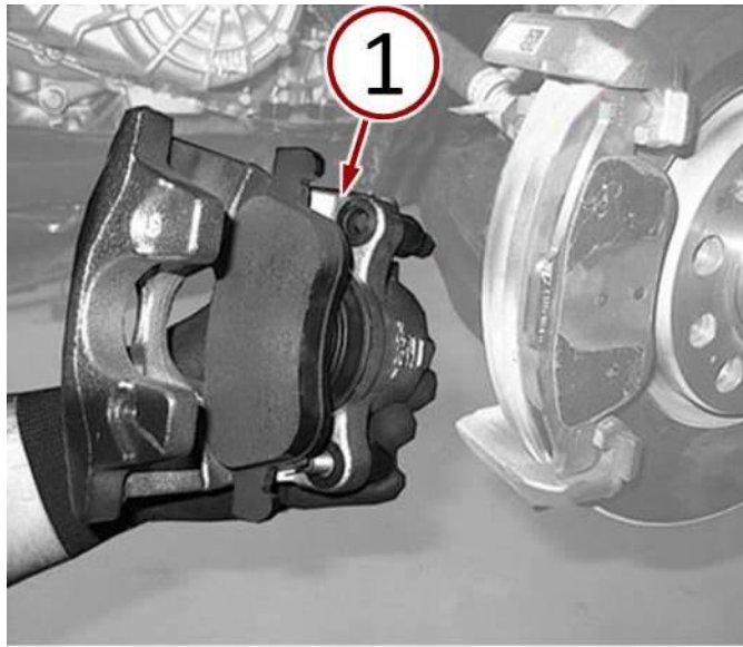
Fig. 9 Install Brake Caliper With Inboard Brake Pad
