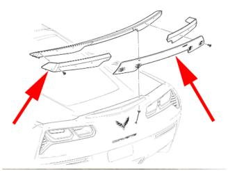
During the installation of the rear wicker bills that are fastened on the rear spoiler, some technicians may revert to the use of power tools to tighten the fasteners.
