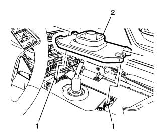
14. Install the upper closeout boot to the transmission control assembly.
