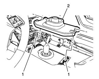
2. Remove the upper closeout boot (2) from the transmission control assembly.
