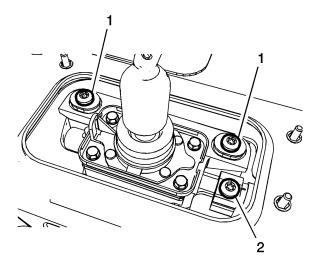
10.6. Tighten the shift control mounting bolts (1) to 30 Y (22 lb ft).
