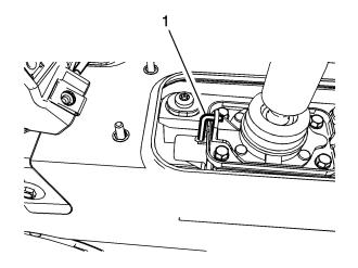
11. Lift to release the shift control neutral lock pin (1).
