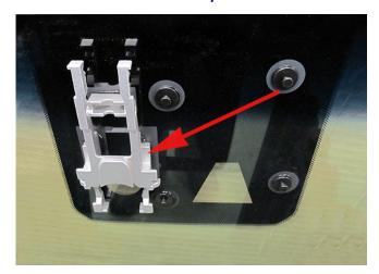
Some customers may comment that the inside rear view mirror or front camera is loose or that the mirror/camera mounting bracket is loose or has fallen off.
