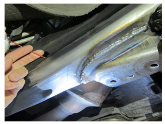
17. Apply a light flash-coat of Lloyds Kryptonite Metal Treatment P/N 36502 Life Long Rust Protection (14 ounce aerosol), or equivalent, to all bare areas of the frame where the wax coating was removed. This first coat should flash in approximately 3-5 minutes. Apply a light flash-coat to the inside of the frame rail using existing access holes, as shown. Insert the straw of the aerosol can as far as possible, and slowly work the straw back out while applying material.
