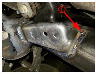
13. Continuous-weld the new bracket into position. Ensure the rear vertical weld (1) is extended approximately 15mm above the edge of the bracket.
