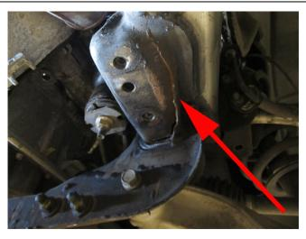
This may be caused by a damaged stabilizer shaft frame bracket. There have been some cases in which the bracket is cracked, as shown. This condition has been found to be the result of insufficient welds between the bracket and frame rail. There have been some cases on older vehicles of corrosion affecting the bracket.
