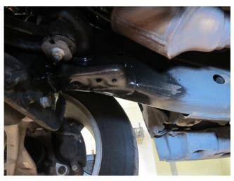
18. Apply a second coat of Lloyds Kryptonite. This can be a heavy coat; double and triple passes with this product, over a light first coat, are not a problem.
