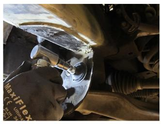
7. After the bracket has been removed, using an angle grinder with 24 grit sand paper or equivalent clean the areas of any excess bracket weld material from the frame so that the new bracket can sit flush in the location of the old one.
