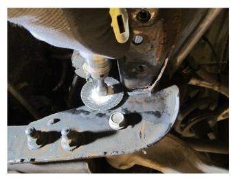
6. After all the wax coating is removed, using a cut off wheel, remove the old bracket from the frame.
