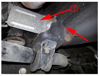
2. Raise the vehicle in the air and inspect the stabilizer shaft frame brackets (both left and right) for any abnormalities or cracks and inspect welds to ensure good alignment and integrity. Refer to Lifting and Jacking the Vehicle in SI.
