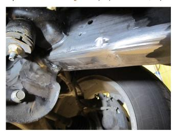
8. Clean the area of all debris in preparation of the new bracket to be welded to the frame.
