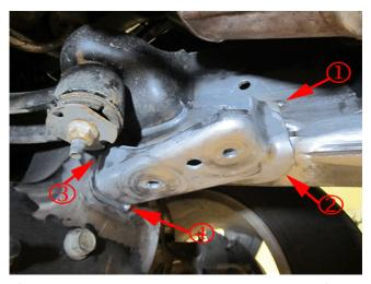
**10.** After the bracket is in location, tack weld the bracket to the frame in all 4 corners of the bracket. This will keep the bracket from moving while welding the bracket fully to the frame.
