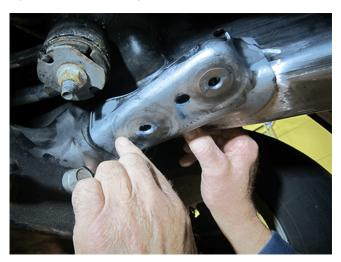
**9.** After the area is clean of all debris, place the new bracket in the location of the removed one. The bracket should seat against the frame crossmember bracket in the most forward position, along the lower surface of the frame rail, and along the inner surface of the frame rail in the rear.
