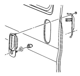
Replace the side sliding door outside handle. Refer to Sliding Door Outside Handle Replacement in SI.
