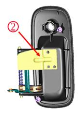
A new handle service part has been released with the elimination of the anti-theft bracket that was on the original part design (1). DO NOT repair the vehicle with a handle containing the anti-theft bracket (2).
