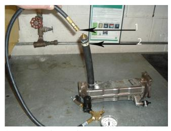
6. Connect the hose fitting (1) of pressure tester J-46091-1 Charge Air Cooler Tester Regulator to the EGR Cooler Hose Adapter (2) on the EGR cooler as shown.
