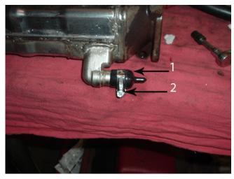
5. Install the Cap Plug(s) (1) and tighten the clamp(s) (2) on the EGR cooler hose barb(s) as shown.
