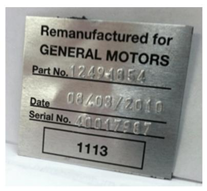
The tag is made of metal and is approximately 2 in x 1-11/16 in (5.1 cm x 4.3 cm). It is installed on all remanufactured for GM service engines and new engines assembled by non-GM suppliers.
