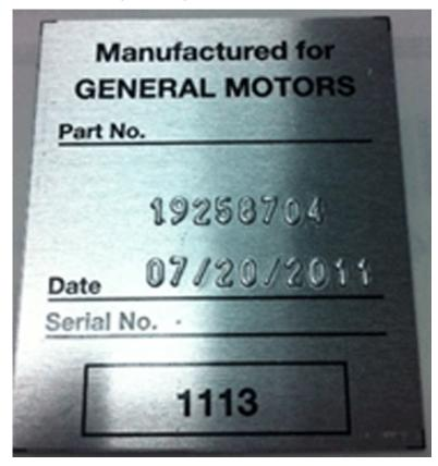
The tag is made of metal and is approximately 2 in x 1-11/16 in (5.1 cm x 4.3 cm). It is installed on all manufactured for GM service engines and new engines assembled by non-GM suppliers.
