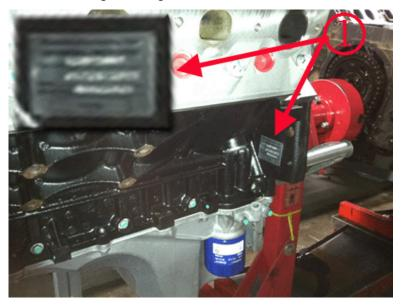
All remanufactured engines have a label on the right or left side of the block. A list is provided below to indicate which side of the block the label may be found for each engine application.
