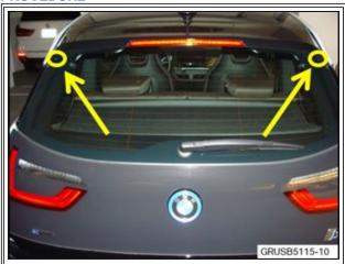
1. Locate the rear hatch spoiler. Look at the clearance gap between the spoiler and glass in these two areas. If the gap is less than 3.2 mm, the buffers stops in the spoiler must be replaced with a new design flat head buffer.
