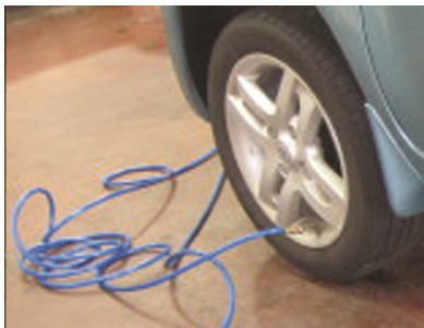
Long heavy hose with Lock-on air chuck or wheel at 6 O'clock position
