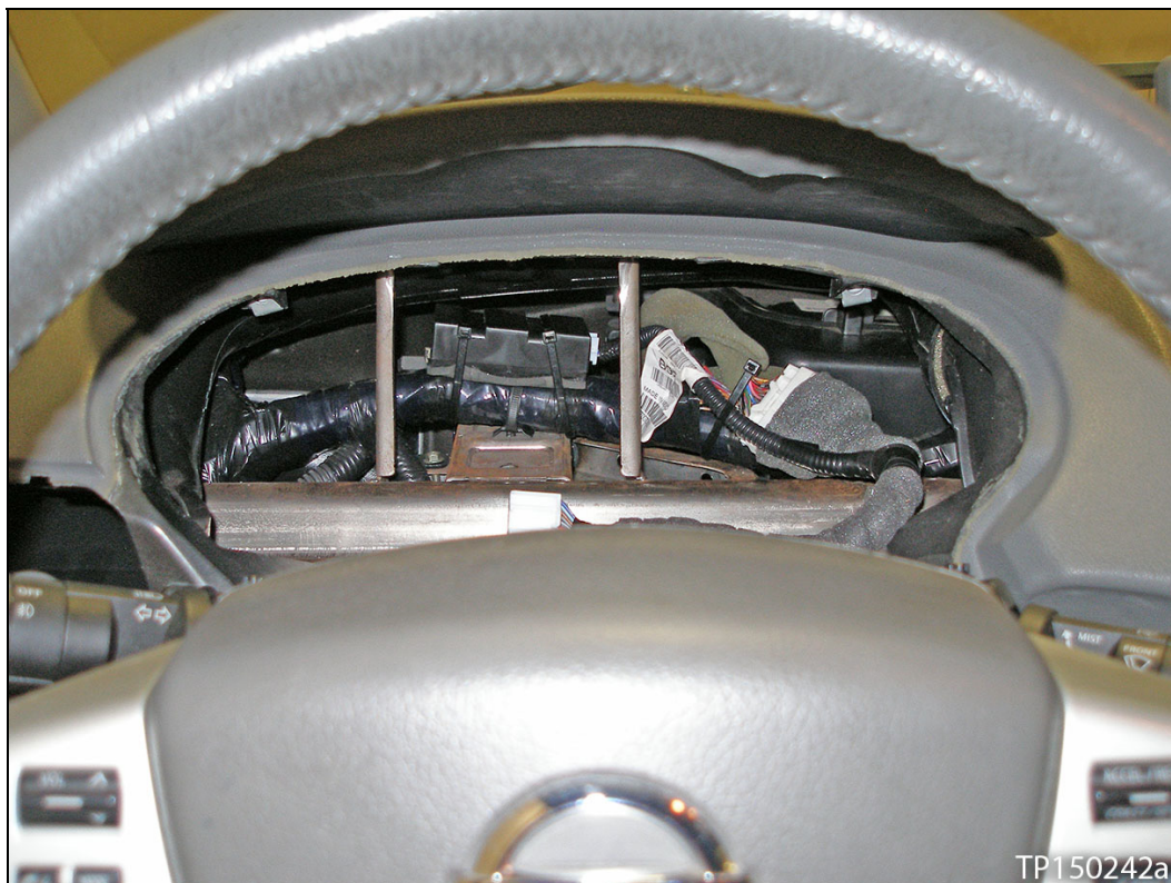
Figure 4: Amp and jumper harness installed
