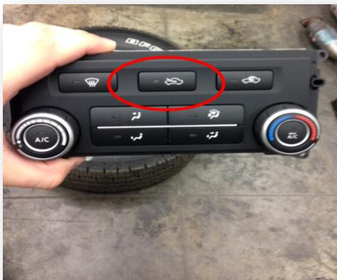
NG: Heated Mirror Switch Missing
