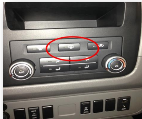
OK: Heated Mirror Switch Installed
