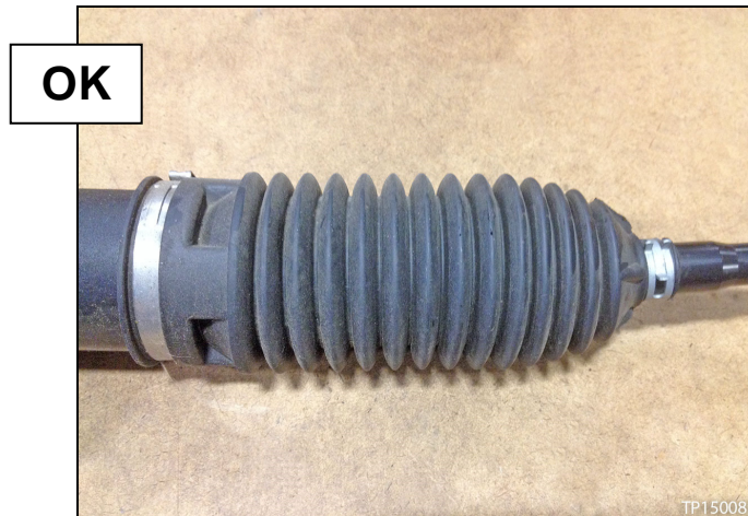
Figure 6: Example of no leaks inside the boot. Boot is dry, dusty, feels firm to the touch.
