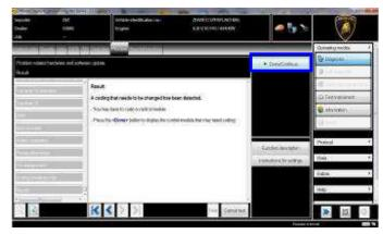
**26.** New coding has been calculated on the 08 – Air conditioning system and must be written in the control unit.
