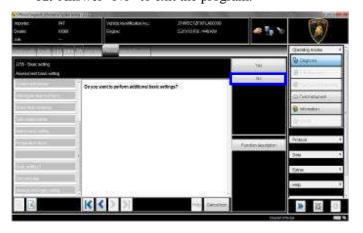
**62.** Chech that all errors are erased on the Air Conditioning control unit. In the case still remain some sporadic errors, erase again.
