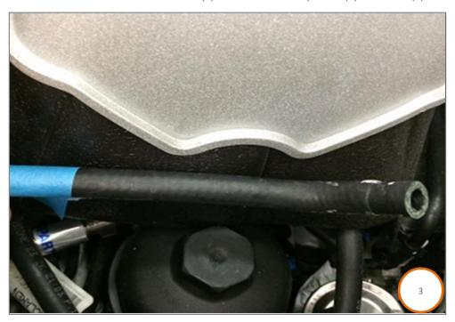
16. Take the new degas hose 11F1468CP and remove the spigot from the new hose (4) the remainder of the hose can be discarded.
