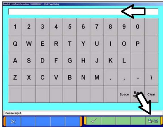
h. Click the icon in the lower RH corner of the screen to have MUT-III automatically read the VIN. If a message appears saying the VIN cannot be input automatically, manually enter the 17 digit VIN into the VIN field at the top of the page. Make sure the VIN is correct and click the check mark.
