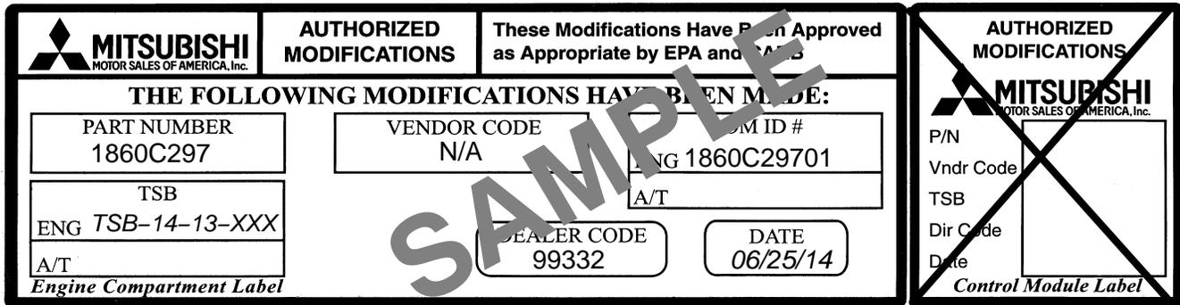
**The Control Module Label is NOT used for this reflash. It should be discarded.**
