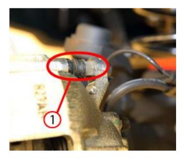
Fig. 2 Caliper Slide Pin Location
