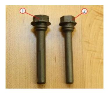
Fig. 1 Caliper Slide Pin Comparison
