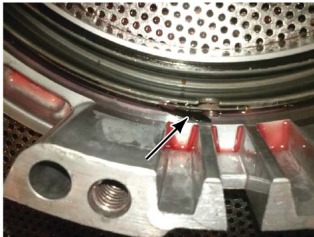
Figure 8. Torn C4 Clutch Piston Seal
