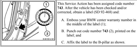
If the vehicle already has a label from a previous Service Action, affix the new label next to the old one. Do not affix one label on top of another one, because a number from an underlying label could appear in the punched-out hole of the new label.
