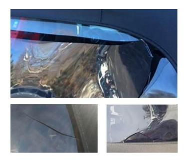
Fig. 1 Examples Of Cracked Vinyl Window - Non Warrantable Condition
