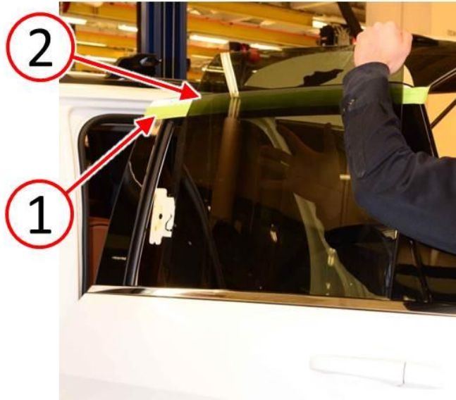
Fig. 22 Install Rear Door Glass
