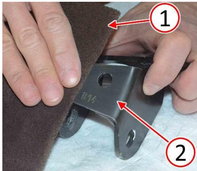
Fig. 6 Scuff Top Surface Of Shock Absorber Bracket With Abrasive Pad
