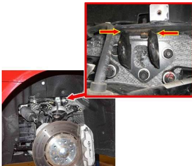
Fig. 1 Noise From Contact Area Between Shock Absorber Bracket And Structure
