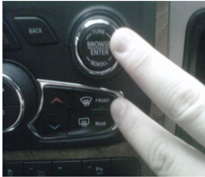
Fig. 2 Take Vehicle Out of Ship Mode
