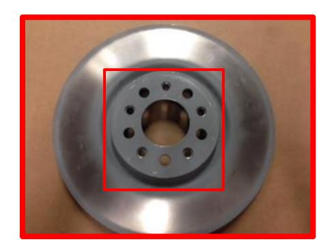
Correct and Suspect parts can be identified by the number of holes on the rotor,
