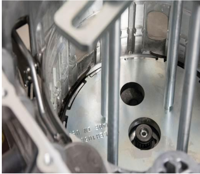
Fig. 11 New Snap Ring Installed
