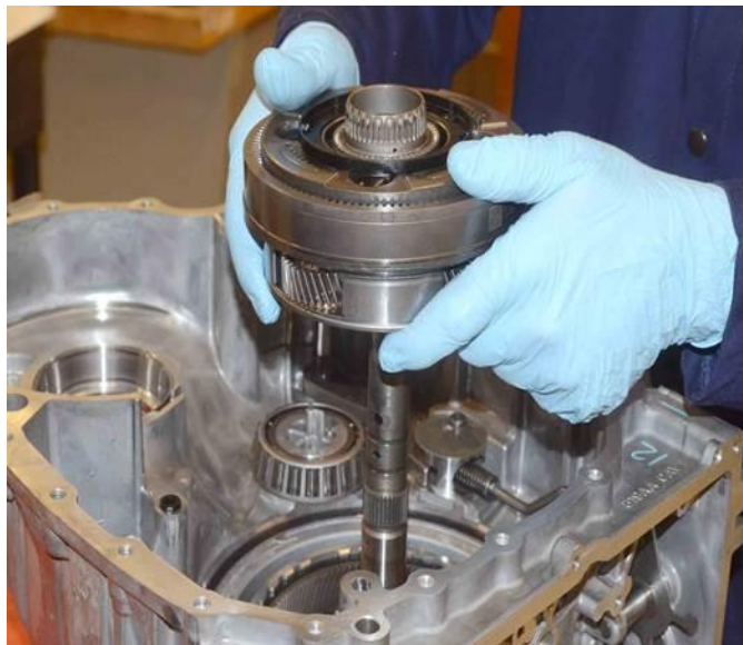
Fig. 15 Gear 4 Planetary Pinion Carrier Assembly
