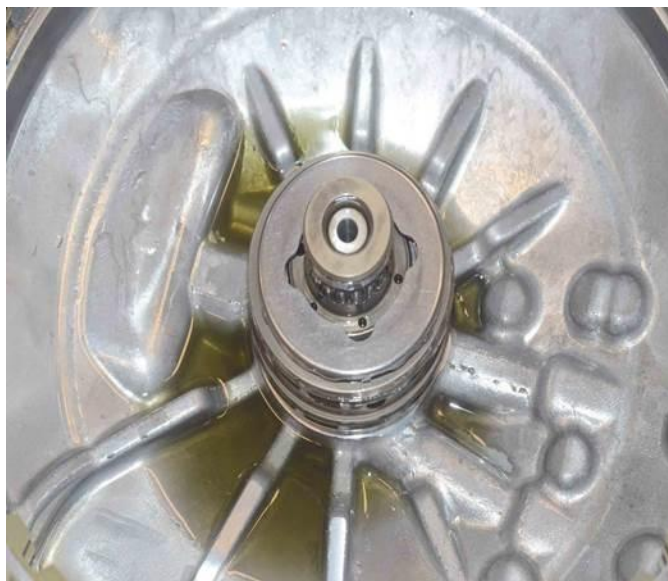
Fig. 12 Thrust Bearing Properly Installed
