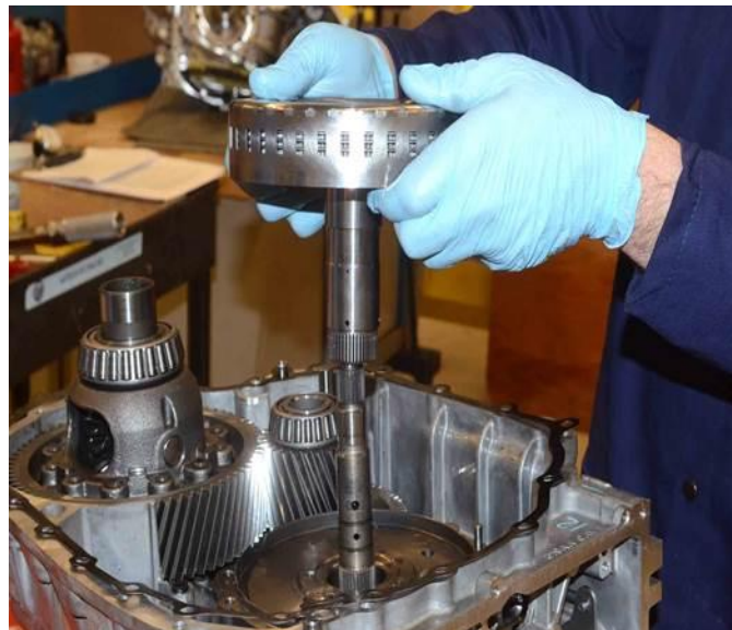
Fig. 19 E Clutch And Hub Installation
