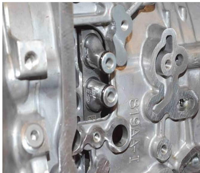
Fig. 25 Transmission Fluid Adapter Tube Orientation
